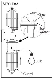
**STYLE#2** - Install specified bulb type and wattage. Install the guard with star washers and nuts.
