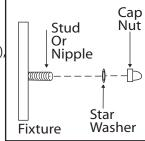
Tuck electrical wires into outlet box and position fixture over studs or nipple on mounting bracket assembly.
